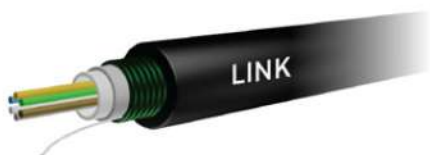
UFC9312A F.O. Outdoor / Indoor, Armored 12 Core, LSZH - FR, OS2
